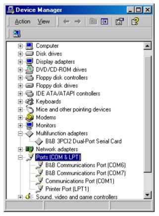
Under **Multifunction Adapters**, the B&B 3PCI2 Dual-Port Serial Card is installed.
